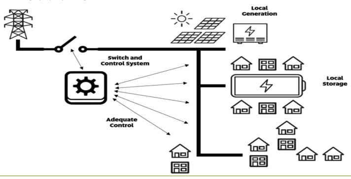
This diagram shows how solar and battery systems on households, community buildings, businesses and at neighbourhood scales together with control systems and disconnection/re-connection switches can all combine to enable our community to be energy self-sufficient, particularly during outages.
